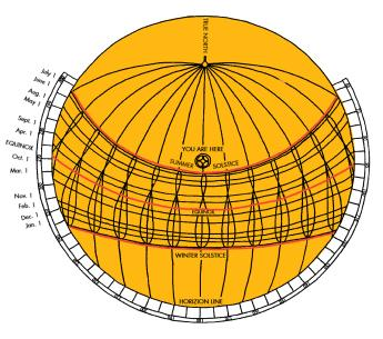
The diagram inlaid on the floor of Visitor Center is the solar observatory or a map of the apparent motion of the sun over the course of the year.
